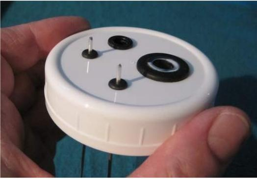
5. Install the Silva-Cap onto the jar. This will require carefully lowering the lid, making sure both rods and the PVC air pump support tube (if installed on your Silva-Cap) enter the water together. Then, carefully turn the jar while holding the lid until the lid is snugly tightened onto the jar.
